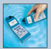
The GPFC<sup>E</sup> measures a dynamic range of free chlorine concentrations wider than the range of colorimetric test kits.
